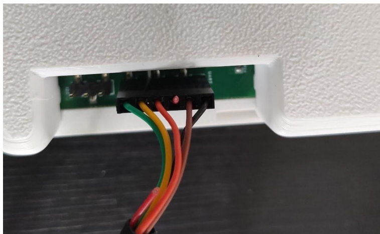
Correct connection on the connector marked “UART”: follow this wire order.
